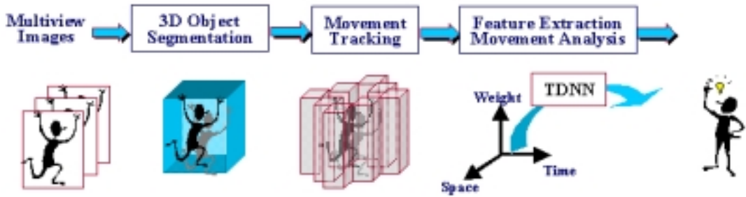
Figure 2. Basic structure for movement tracking and analysis using vision-based 3D interface. In the proposed vision-based 3D interface, an object is segmented out from background scene and then movement is tracked by observing the invisible 3D boxes in the segmented user’s personal space. The movement features, extracted based on the Laban’s movement theory, are mapped to meaningful symbols by time-delay neural networks.
