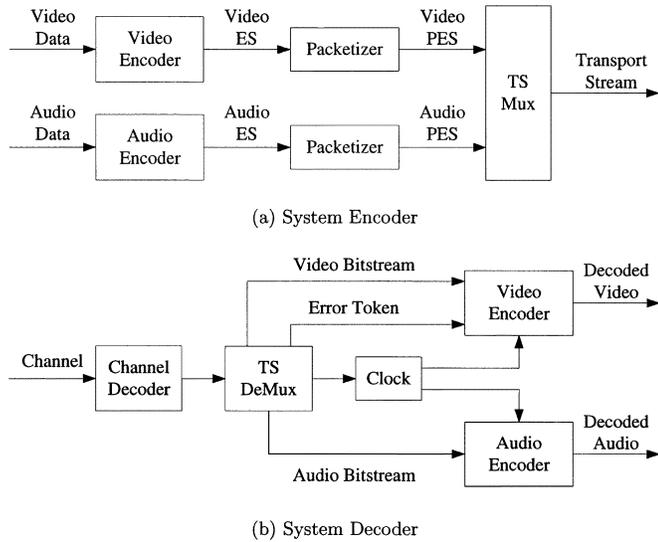
Fig. 1. MPEG-2 TS system for noisy channel.
