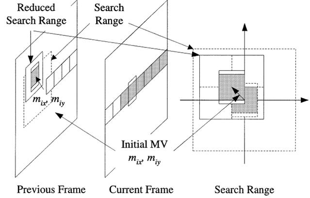
Fig. 4. EMA with Initial Motion Vector (IEMA).
