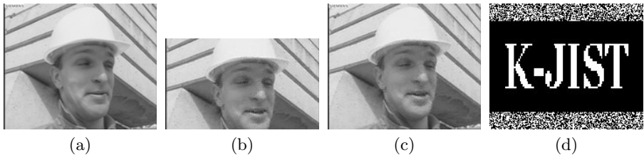
Fig. 9. Experimental results to frame cropping : (a) the watermarked frame, (b) the cropped version of (a), (c) the replaced version, (d) the extracted logo image
