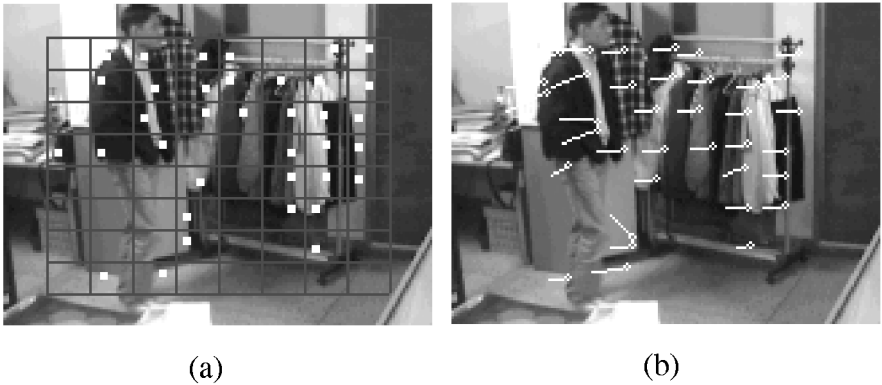
Fig. 2. Block-based Motion Estimation (a) the selected 9x9 region for block motion estimation (b) the extracted block vectors
