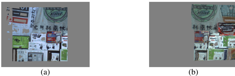
Fig. 2. Projected images (a) projection of 3D point cloud of destination view onto its own view (b) projection of 3D point cloud of source view onto destination view
