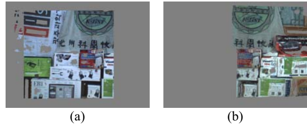
Figure 4. Projection of 3D point cloud onto image plane (a) projection of 3D point cloud of destination view onto its own view (b) projection of 3D point cloud of source view onto the destination view
