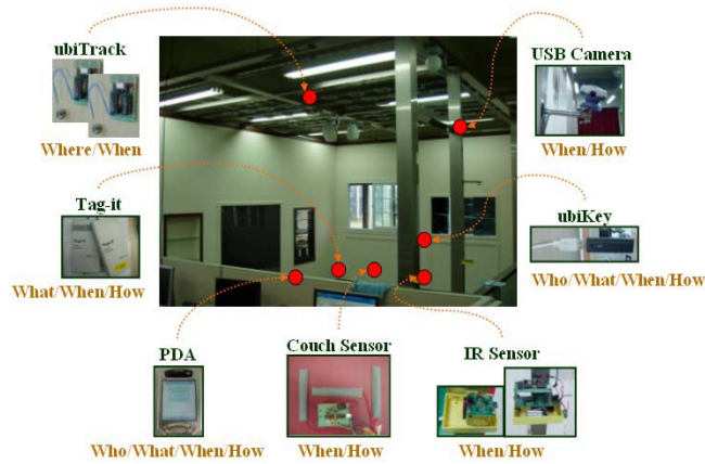
Fig. 1. ubiHome test-bed with various sensors
