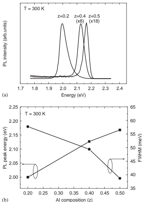
Fig. 2. (a) 300 K-PL spectra of digital-alloy  $\text{In}_{0.49}(\text{Ga}_{1-z}\text{Al}_z)_{0.51}\text{P}$  grown at 425 °C as a function of Al composition ( $z$ ). (b) PL peak energy and line width of digital-alloy  $\text{In}_{0.49}(\text{Ga}_{1-z}\text{Al}_z)_{0.51}\text{P}$  as a function of Al composition ( $z$ ).
