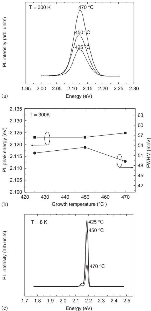
Fig. 3. (a) 300 K-PL spectra of digital-alloy  $\text{In}_{0.49}(\text{Ga}_{0.6}\text{Al}_{0.4})_{0.51}\text{P}$  as a function of growth temperature. (b) PL peak energy and line width of digital-alloy  $\text{In}_{0.49}(\text{Ga}_{0.6}\text{Al}_{0.4})_{0.51}\text{P}$  as a function of growth temperature. (c) 8 K-PL spectra of digital-alloy  $\text{In}_{0.49}(\text{Ga}_{0.6}\text{Al}_{0.4})_{0.51}\text{P}$  as a function of growth temperature.
