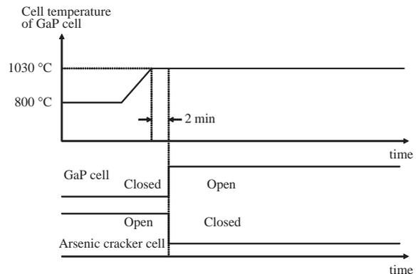
Fig. 1. Sequences of cell temperature and shutter for no parasitic contamination between phosphide and arsenide.
