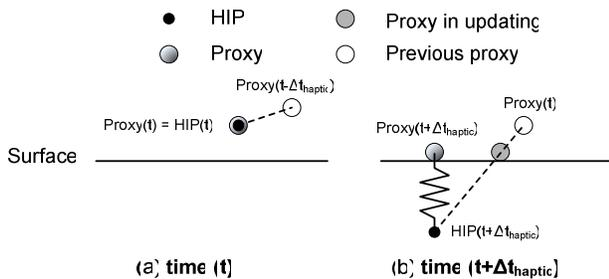
Fig. 3. Typical proxy-based haptic rendering algorithm with plane surface.
