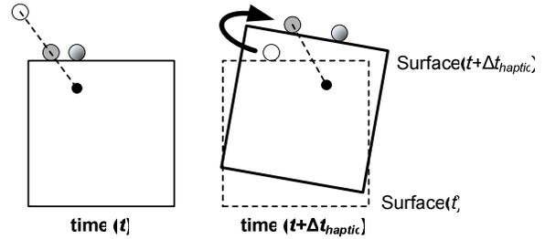
**Fig. 6. Collision detection correction in a proxy-based algorithm with a rigid-body object.**
