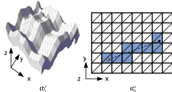
Fig. 4. (a) Height field topographic map. (b) 3D side view. (c) Top view and local search for collision detection.
