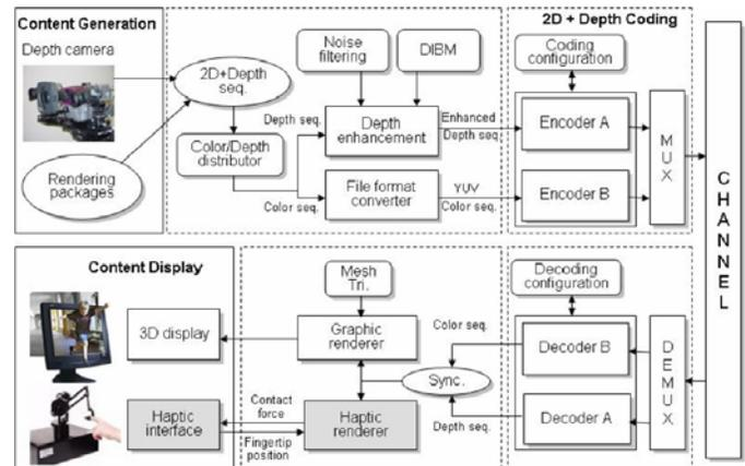
Fig. 2. Overall system architecture for a haptic interaction enabled 3D video player system.
