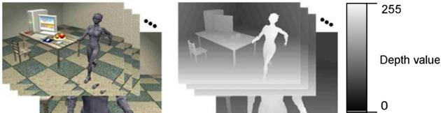
Fig. 1. General color video and synchronized depth video.
