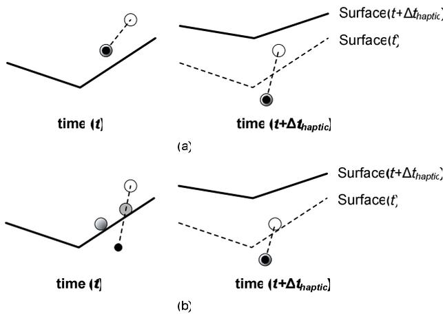
**Fig. 5. Collision detection failure of the proxy graph algorithm with depth video (y-direction view of the depth video surface).**
