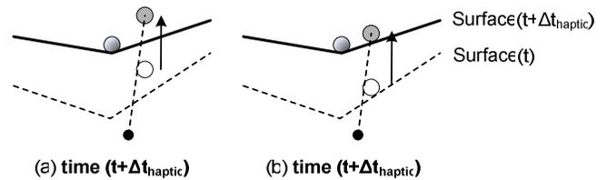
**Fig. 7. Correction of the previous proxy position by the amount of surface movement.**
