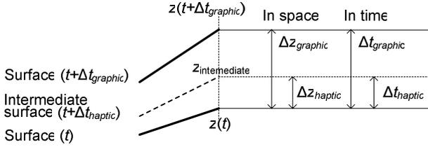
**Fig. 8. Intermediate surface interpolated between the current surface and the next buffered surface**
