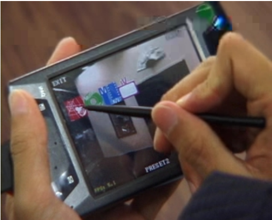
Figure 1. In this figure a PDA is a Universal Control(ubiController) for simulating sensors.
