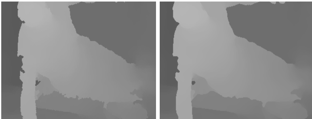
Fig. 7 Depth Comparison (left: original depth, right: 7x7 median-filtered depth)
