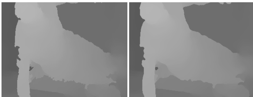
Fig. 4 Depth Comparison (left: original depth, right: 7x7 median-filtered depth)
