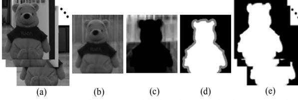
**Fig. 1.** Matting procedure. (a) Multi-view images, (b) SAI, (c) Variance image, (d) Trimap, and (e) Multi-view alpha mattes.
