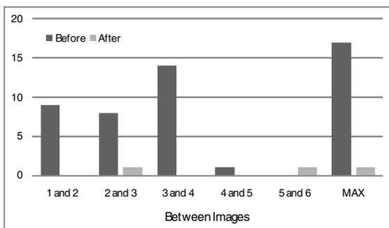
**Fig. 12.** Vertical Mismatch in Pixels between Images
