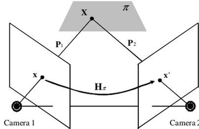
Fig. 3. Point Transfer via the Plane  $\pi$
