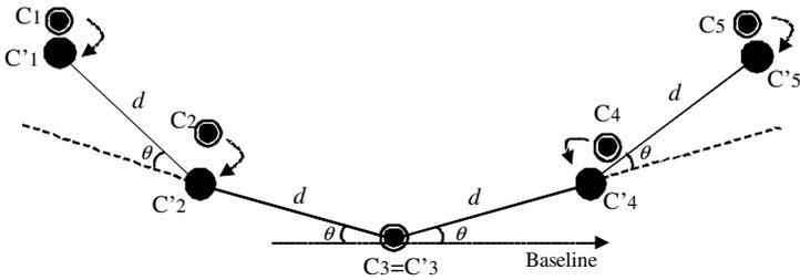
**Fig. 6.** Finding New Camera Centers for Odd Number of Cameras
