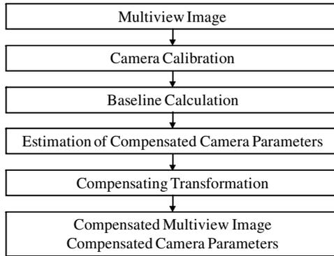
**Fig. 4.** Geometrical Compensation for an Arc Multi-Camera Array
