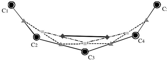
**Fig. 5.** Iterative Midpoint Connection
