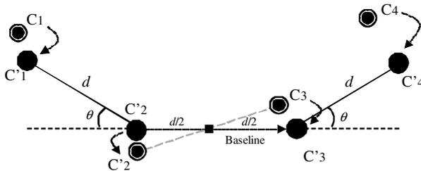
**Fig. 7.** Finding New Camera Centers for Even Number of Cameras
