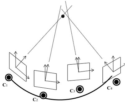
**Fig. 2.** A Practical Arc Multi-Camera Array
