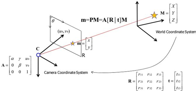
Fig. 1. Pinhole Camera Model
