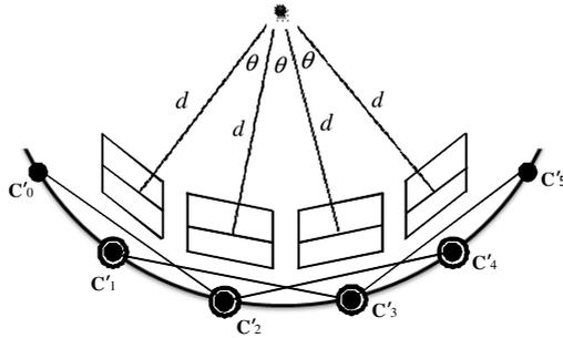
**Fig. 8.** Compensated Arc Multi-Camera Array
