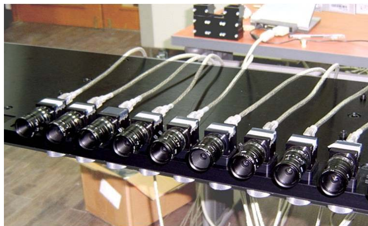
Figure 1: Nine-view camera system
