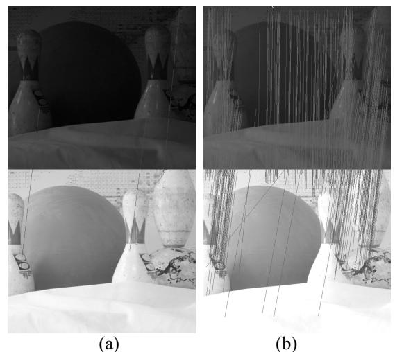
Figure 2. Results of the feature-based matching process (a) without and (b) with the histogram equalization
