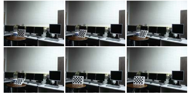
(b) Relative calibration of the right camera
