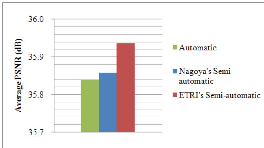
Fig. 2. Objective quality of the synthesized view for EE1
