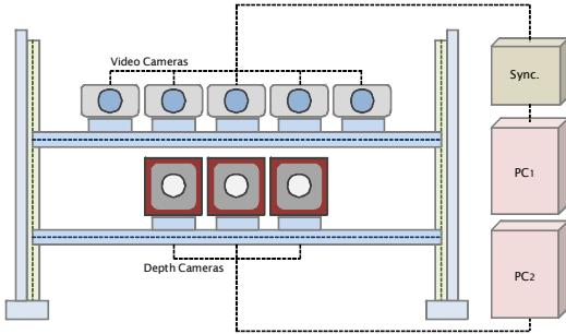
**Fig. 1.** Multiple color and depth cameras
