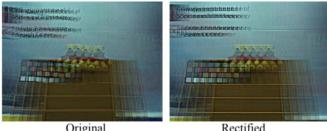
Fig. 7. Result of multi-view image rectification
