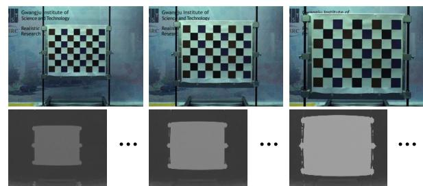
**Fig. 6.** Images for depth calibration
