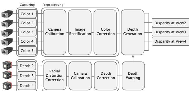
**Fig. 3.** Procedure of the proposed method
