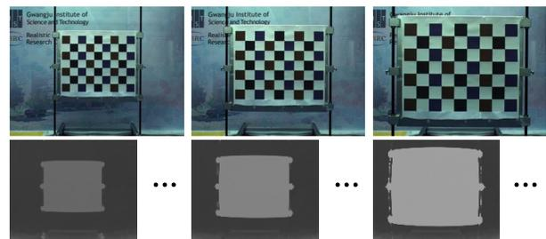
Fig. 6. Images for depth calibration
