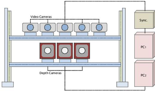
Fig. 1. Multiple color and depth cameras
