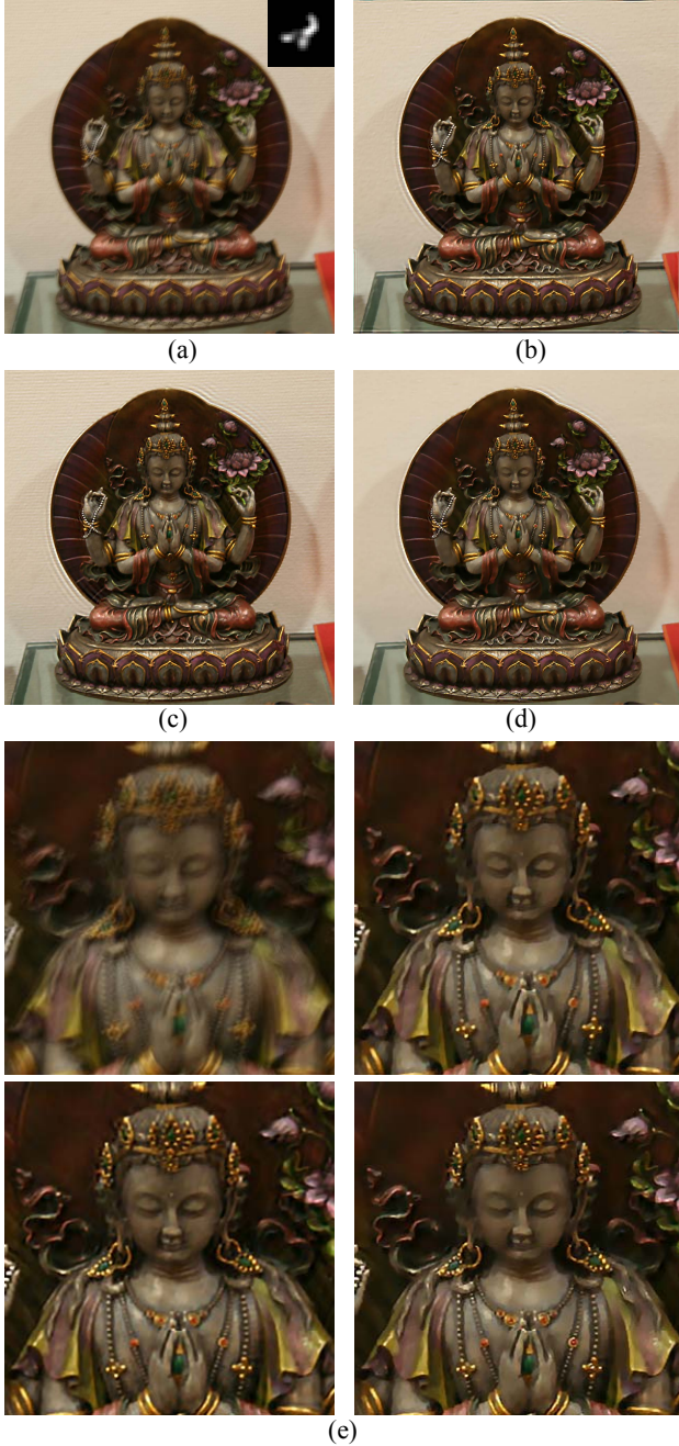
Figure 7: Statue. (a) Blurred image and estimated kernel. (b) TV regularization. (c) Levin et al 's method. (d) Our method. (e) Close-up views of (a)-(d).
