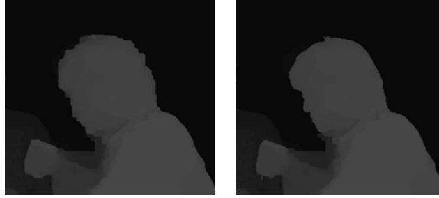
Fig. 3. Post-processing using bilateral filter: depth map by DERS 5.0(left), refined depth map(right)
