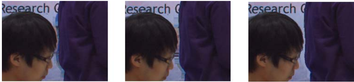
(a) Synthesized image for 81 st frame of Café_3 by: the inpainting method in general mode (left), the hole filling method in BNR (center), the proposed method (right)
