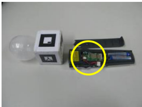
Fig. 12 The internal components of the manipulation tool included a vibration actuator, a Bluetooth communication module, and a microcontroller
