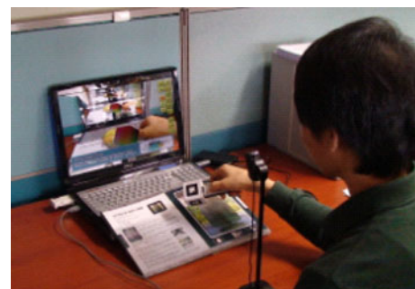
Fig. 3 Running environment of Digilog Book viewer; the monitor, camera, and book were aligned
