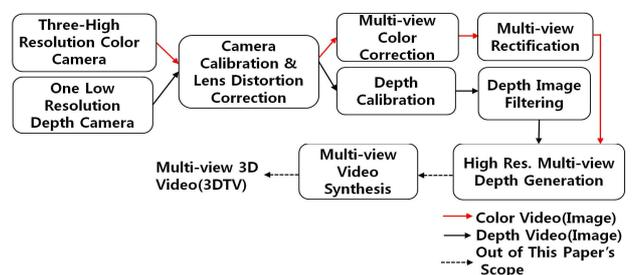
Figure 1. The overall framework of multi-view 3D video acquisition
