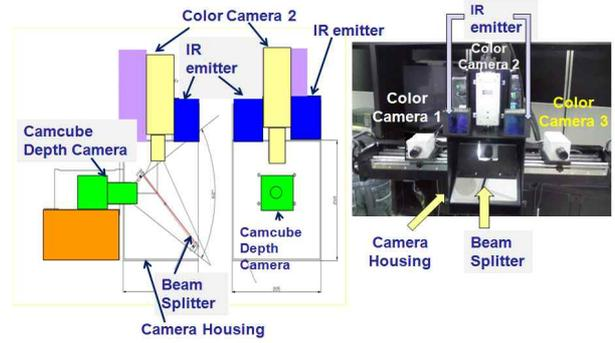
Figure 2. The structure of the proposed hybrid camera system
