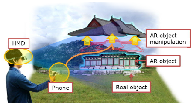
Figure 1. A user is wearing a HMD and grasping a mobile phone to manipulate 3D object in AR environment.
