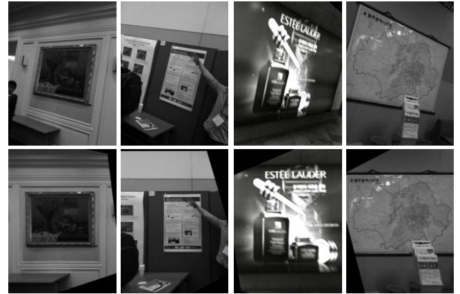
Fig. 2. Image rectification results using vanishing points
