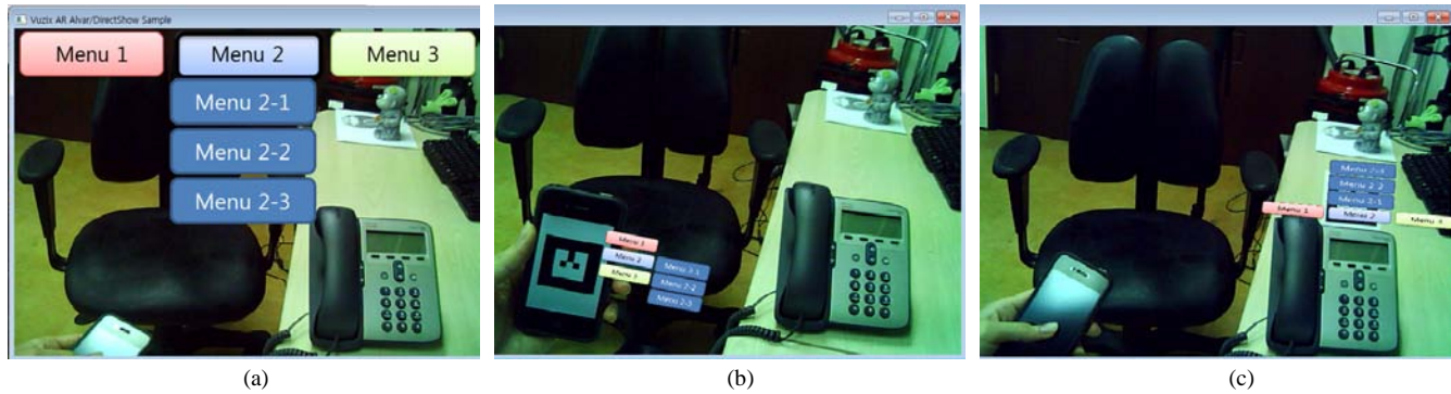
Figure 3. Three menus on focusable location(implemented): (a) display-referenced, (b) manipulator-referenced, and (c) target-referenced.
