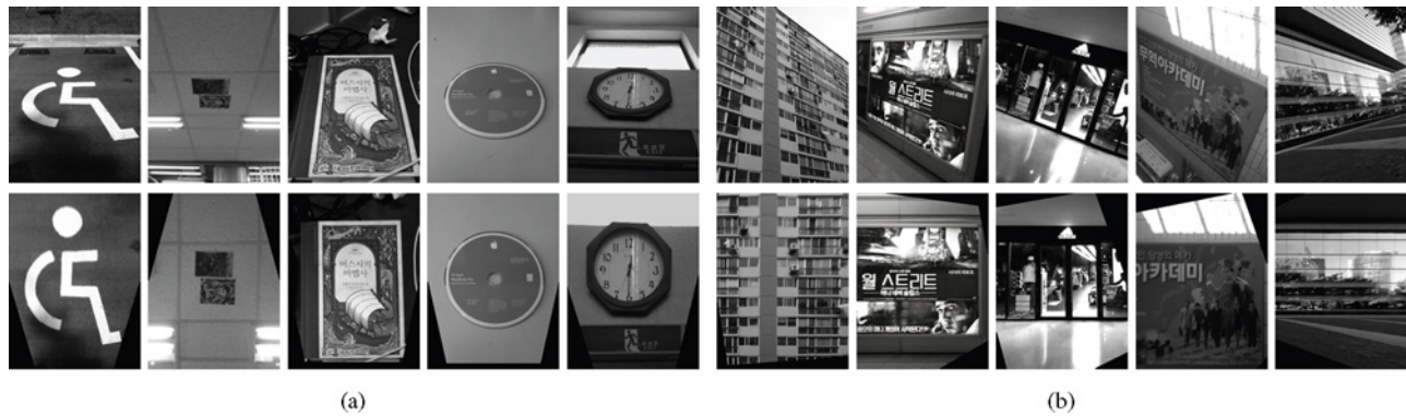
Fig. 8. Examples of estimated fronto-parallel views (bottom row) from different input images (top row). (a) Only the phone accelerometers are needed for horizontal surfaces (columns 1–4). It is also true when a vertical surface is rotated in pitch only, as shown in column 4. (b) However, for slanted vertical surfaces, we need to combine the accelerometer’s output with vanishing points detection.
