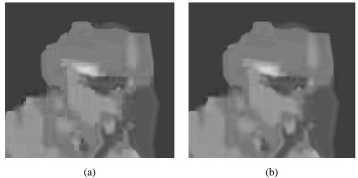
Figure 4. Result of deblocking filtering: (a) Before deblocking filtering, (b) After deblocking filtering
