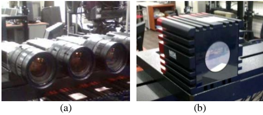
Fig. 2. Multi-camera and TOF depth sensor (a) three color video cameras (b) SR4000
