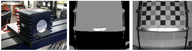
(a) SR4000 (b) Depth map (c) Intensity map Figure 1. TOF depth camera and captured images
