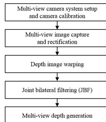
Fig. 2 Overall procedure of multi-view depth generation
