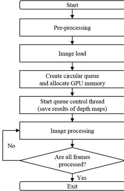
Fig. 3 Overall procedure of proposed multi-view depth generation method
