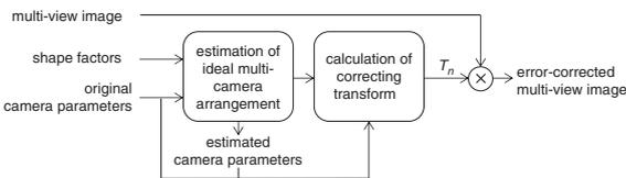
**Fig. 2** Procedure of proposed geometric error correction
