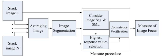
Fig. 1 Procedure of the proposed method
