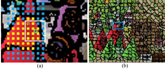
Fig. 3. Superpixel-based smooth filter. Green pixel is center pixel p , yellow pixels have the same label with center pixel q , and blue pixels have the different label with center pixel q .
