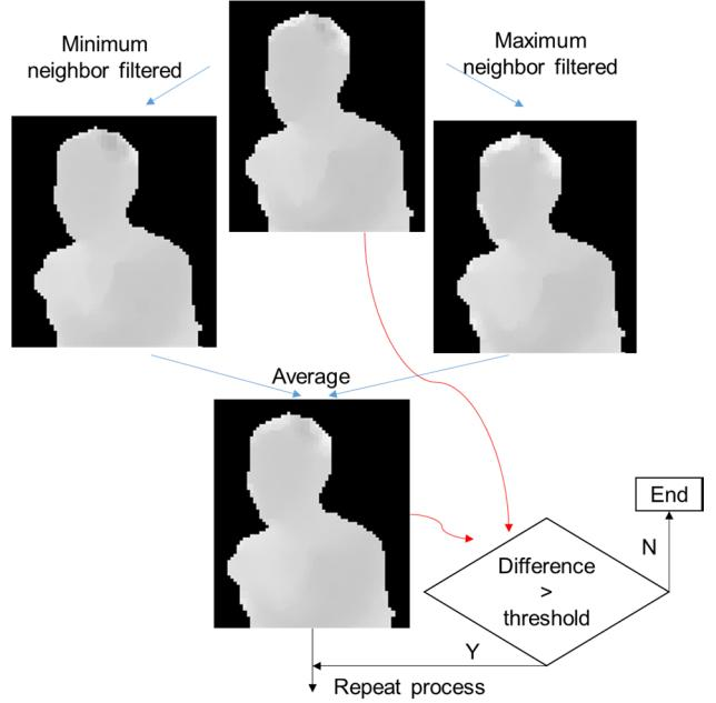
Fig. 5. Iterative averaging of minimum and maximum neighbor filtered images.
