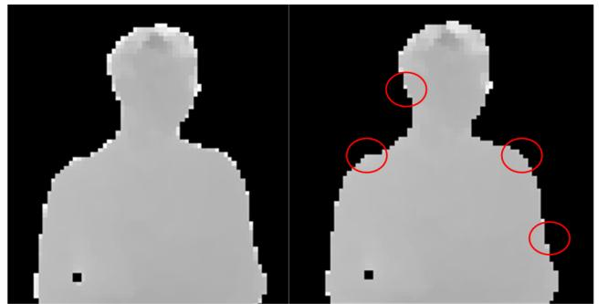
(a) Before boundary filtering      (b) After boundary filtering
