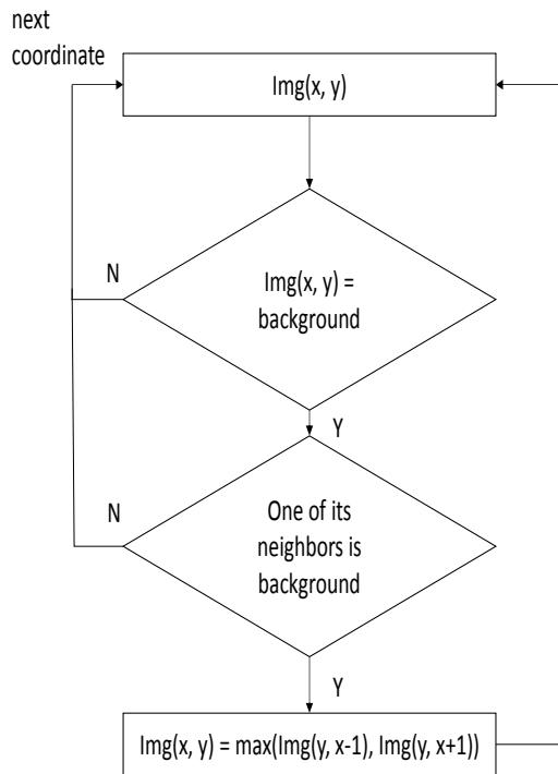
Fig. 2. Flowchart of object boundary filtering in the horizontal direction.
