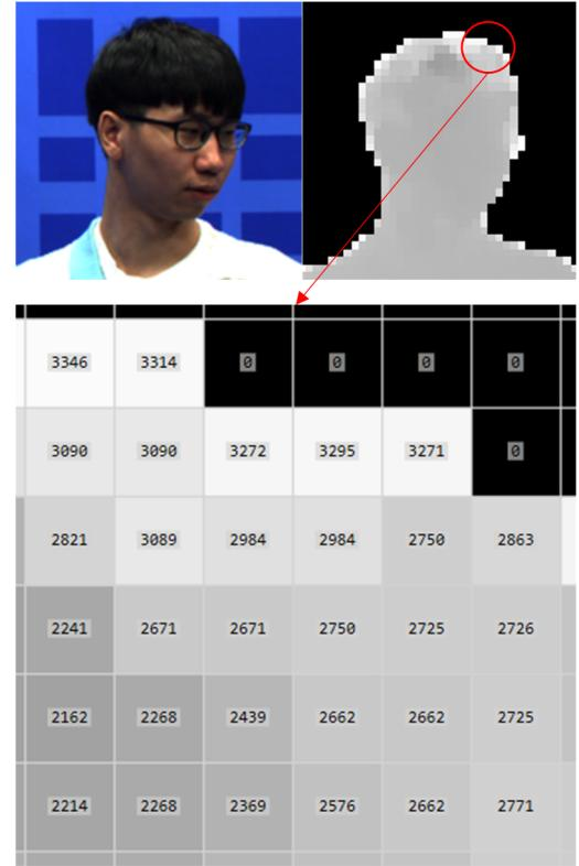
Fig. 1. Inaccurate distance data within a foreground object.
