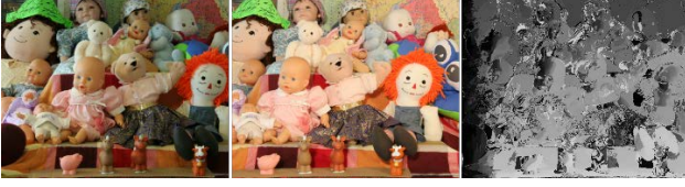
(a) Left view (b) Right view (c) Disparity map Figure 1. Stereo matching result under the radiometric variation
