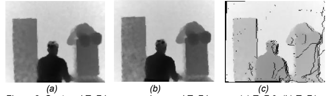
Figure 3. Captured ToF images and warped ToF image : (a) ToF 0; (b) ToF 1; (c) ToF0-to-ToF1 warped image
